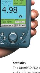
The LaserPAD PDA can perform complete statistical and power trend analysis for stability and drift measurements. From 40 to 2000 data points can be recorded and analyzed over a selected period of time for display on a strip chart or histogram plot.
